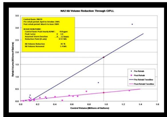
Fig 1. Flow Data from CIPP Project
