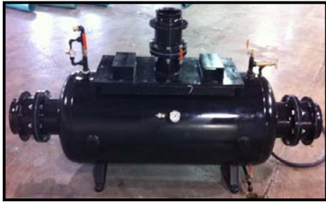
Figure 2: Hydrostatic Test Tank (as built)
