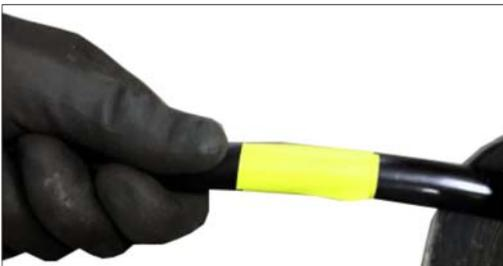
Attach a visual marker (tape) to the outer casing of the flexible shaft. Place it around half a meter from the end point of the shaft. The mark will indicate the chain's location and prevent possible injuries when a tool is removed from the drain, including injury by rotating parts.
