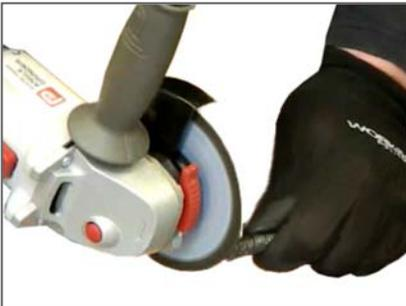
Always inspect the flexible shaft before each use. If there are potential weak points or the shaft is damaged, cut off the damaged length using an angle-grinder. This should be done outside in a clear area as there will be sparks generated by the process.
