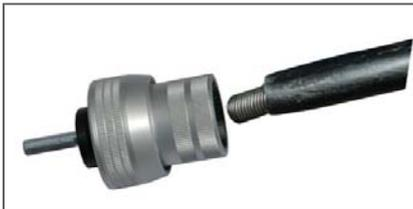
The shaft rounder smooth's the end of the flexible shaft, preventing the user from being cut by the otherwise sharp metal edge .
