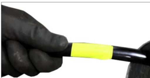
Attach a visual marker (tape) to the outer casing of the flexible shaft. Place it around half a meter from the end point of the shaft. The mark will indicate the chain's location and prevent possible injuries when the chain is removed from the drain, including injury by rotating parts.
