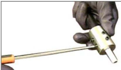
Feed the shaft through the socket to the end and **securely fasten**. The outer casing should reach all the way to the base of the shaft socket to protect the shaft.
